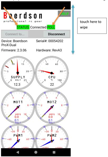
As you drive your model, the data is continuously updated and the pointer instruments display the data.
