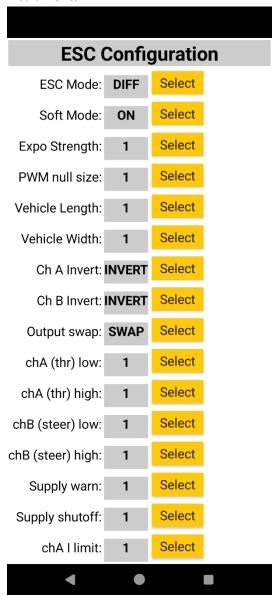
The respective name of the paramter is listed on the left, the value currently stored in the ESC is displayed in the middle, and on the right there are buttons that you can use to select new values. Once you have made the desired
